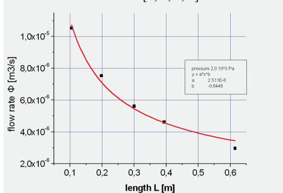
Fig. 5: Flow rate  $\Phi$  as a function of the length of tubes of  $R = 0.88$  mm.
