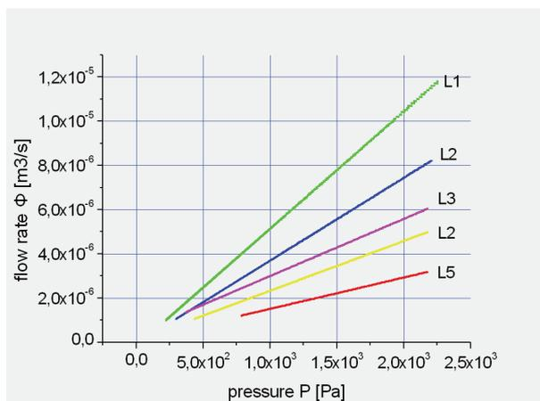
Fig. 4: Flow rate  $\Phi$  as a function of the pressure  $P$  for tubes of  $R = 0.88$  mm and different lengths,  $L$ .
