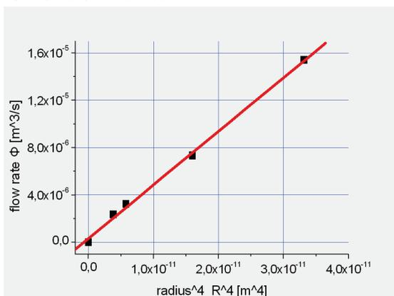
Fig. 7: Plot of the flow rate,  $\Phi$ , as a function of the forth power of radius, for tubes of equal length (0.30 m) and of the same solution.
