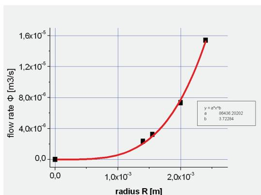
Fig. 6: Plot of the flow rate,  $\Phi$ , as a function of the radius, for tubes of equal length (0.30 m) and of the same solution.
