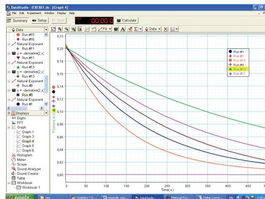
Fig 3b: The print screen with fitted curves of the heigth vs time for finding the function of the derivate and the flow rates.
