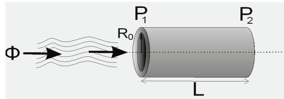
Fig 1: Voluminal laminar flow  $\Phi$  of uniform viscous liquid through a cylindrical tube with the constant circular cross-section.
