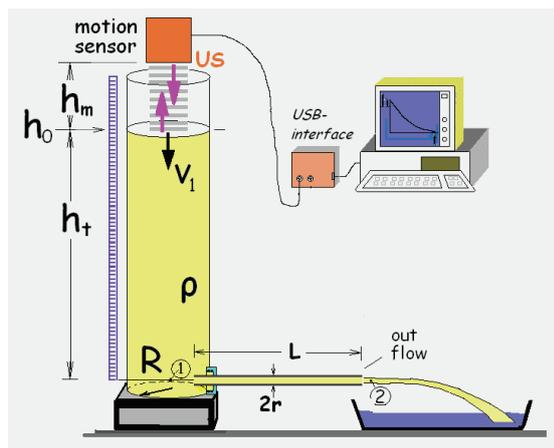
Fig. 2: A schematically draw of the experimental set up used for the measurements
